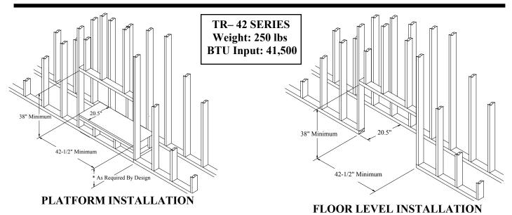
The above framing diagram does not show a hearth. A hearth is not required, but often used with this appliance. If a hearth is desired, it must be constructed so as not to inhibit the valve access door at the bottom of the appliance. The hearth need not conform to codes applicable to solid fuel appliances.
