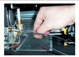
13. Use a small wire tie to secure the blower wiring so it cannot get caught or rub against the fan blades or touch the top of the valve chamber.
