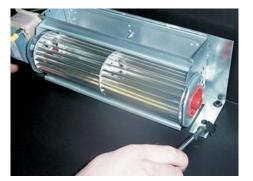
Slide the blower to the rear of the valve chamber, between the two tabs bend up in step #2. With the blower in place, bend the tabs tight onto the blower.
