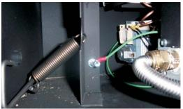
12. Attach the ground wire to the left side firebox support in the valve chamber. Use a star washer in both the front and back of the ground terminal. Use (1) coupling nut to secure the terminal.
