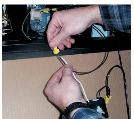
Connect the white rheostat wire to the black lead from the blower. Connect the black rheostat wire to black lead from the blower power cord. Fasten with yellow wire nuts.
