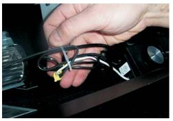
14. Use a small wire tie to secure all loose wiring near the rheostat.
