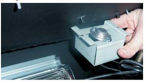
10. Secure the heat sensor to the two studs located at the top of the valve chamber
