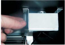
11. Use (2) coupling nuts to attach the sensor to the studs.
