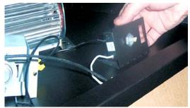
8. Install the rheostat in the bracket and secure with the nut. Put the knob on the rheostat.
