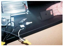
7. Locate the rheostat bracket in the front right hand side of the valve chamber. Bend up to approx. 80-85 degrees.
